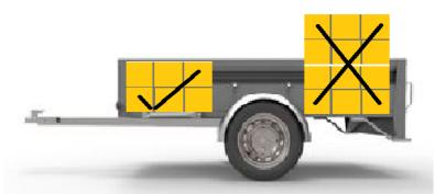
In the above image, the blocks to the front of the vehicle are not required to be strapped because they do not exceed the height of the sides of the vehicle. The blocks to the rear of the vehicle must be restrained as they exceed the height of the vehicle sides – even if the blocks themselves are strapped. The image below shows the correct method.
