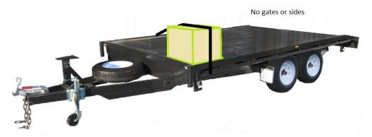
Vehicles with sides may have to have the load restrained depending on the height of the load. If the height of the load is greater than the sides of the vehicle then the load is required to be strapped to the vehicle. See diagram below:
